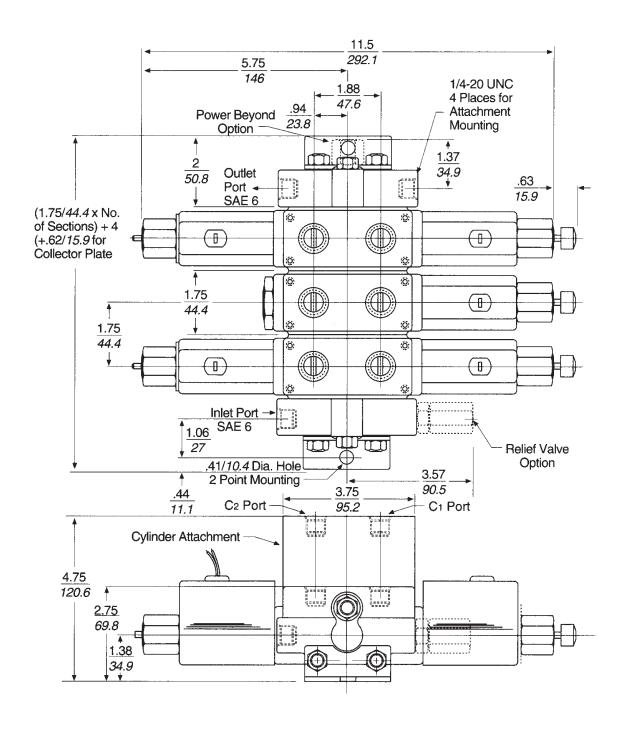
DIMENSIONS ARE IN INCHES (MILLIMETERS) AND ARE FOR REFERENCE ONLY.
